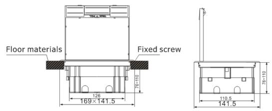
F. G. H>30mm can use longer fixing screws.
