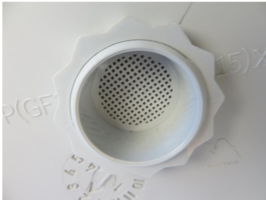
unsignificant penetration of dust around the fitting
